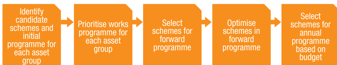
Figure 6 – Developing a Programme of Works
